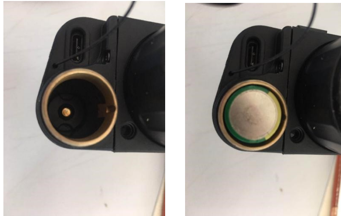
Fig. 5-1 Schematic diagram of battery installation
