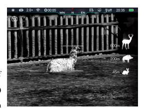
the measurement line to ensure that the measured object is within the line. When you adjust the width of the measurement line, the rangefinder data on the right changes accordingly.
