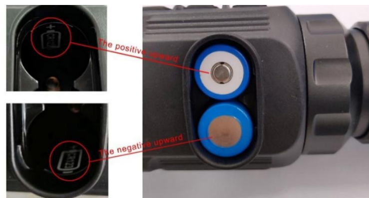
Fig. 8-1 Schematic diagram of battery installation
