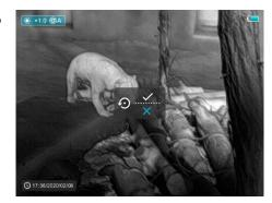
Select the option ' ✓ ' to reset to factory settings or ' X ' to cancel with the Up (5) / Down (6) button. Confirm your selection with a short press of Menu button (4).
