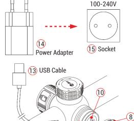
and the LED indicator **(10)** on the device is red. When the indicator **(10)** turns green, it indicates that charging is complete.
